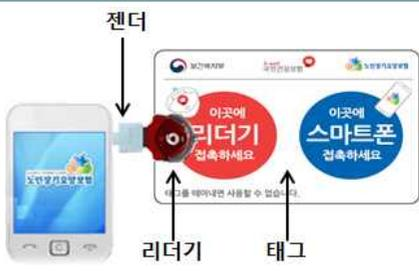
The diagram shows a feature phone on the left connected to a red circular '리더기' (reader) in the center. To the right of the reader is a blue circular '태그' (tag). A sign in the background has text: '이곳에 리더기 접촉하세요' and '이곳에 스마트폰 접촉하세요'. Below the sign, it says '태그를 확인하면 사용할 수 있습니다.' Labels '젠더' (gender) and '리더기' point to the phone and reader respectively.
